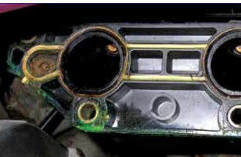
Non-Head Coolant Loss - Leaking inlet manifold gasket.
