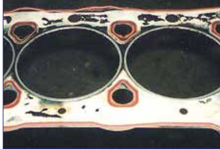
Failed SLS gasket
