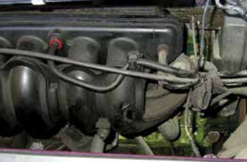
Non-Head Coolant Loss - Green coolant on block from inlet manifold leak
