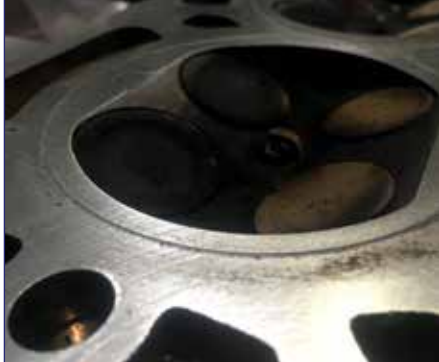
Fire ring indentation - head harness too soft.
