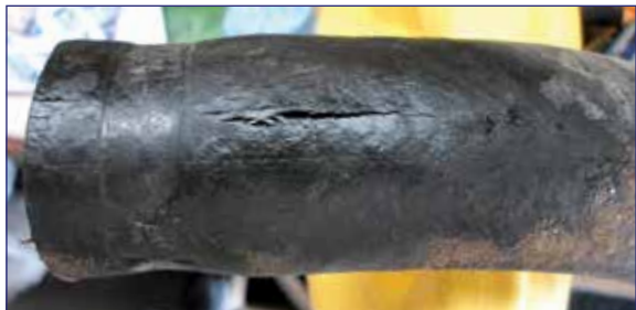
Non-Head Coolant Loss - Perished radiator hose.
